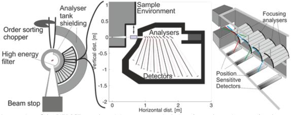
An overview of the BIFROST sample and detector areas, including the analyser-detector chamber (left); a vertical cut of the secondary spectrometer tank (middle); and a cross-section of one multianalyser-detector module (right). IMAGE: BIFROST instrument proposal
