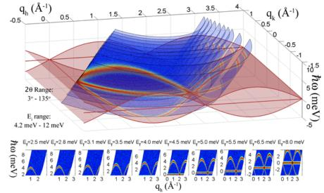
Simulation of data from a single BIFROST data acquisition, using a system with an elastic line and a magnon. Ten surfaces are shown, corresponding to 10 analyser-detector groups. The lower panel shows the 10 individual datasets. IMAGE: BIFROST instrument proposal
