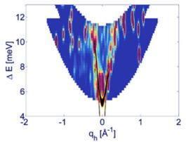
A measurement of an actual sample (YMnO3) made on the MARS spectrometer at PSI with the CAMEA prototype installed, together with theoretical predictions of where the signal should be. The results include high noise levels because of limited neutron intensity. This corresponds to less than 1% of what BIFROST at ESS will record in two seconds. IMAGE: Jonas Okkels Birk
