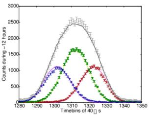
A comparison of the simulation data (solid lines) and the prototype test data (crosses) demonstrating how BIFROST will be able to split the signal of reflected neutrons from a single analyser (grey) into three different energies (blue, green and red). IMAGE: BIFROST instrument proposal
